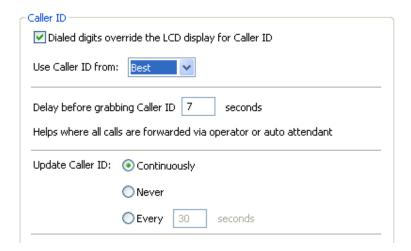
The Recorder software reads the data for Caller-ID from one of the lines on the display. You can vary which line by selecting the option above. If you find that you are capturing other information that appears on the telephone, i.e. a timer, or extension number, you may want to extend the delay timer and perhaps change the option from update continuously to update 'Never'.
