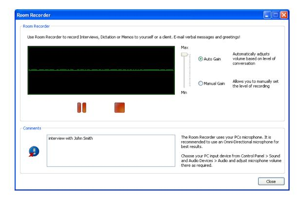
**Room Recorder**, when activated, switches the Recording Source from the Telephone to the user's mic on their PC. This allows for Live Interview recordings, Dictation and many other uses. It is recommended that an Omni-directional mic be used in this case. The auto gain control provides consistent recording results in most cases.
