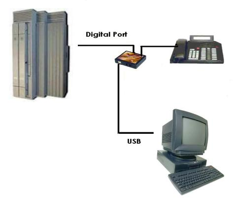
The Xtension Recorder hardware simply connects in-line at the telephone users desktop. No power is required and because the in-line connection is simply a metallic wiring of the 'in' and 'out' connections, Xtension Recorder does not affect in any way the telephone operation with or without connection of the host PC via USB.
