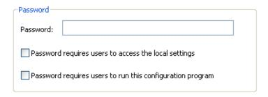
The above option for accessing Local Settings eliminates the ability for the user to access the Options View of the software. This prevents them from changing any and all options that are preconfigured.
