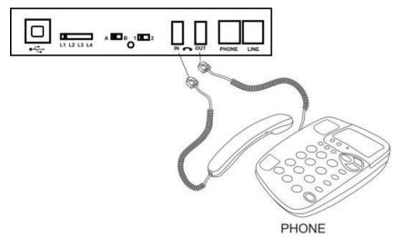
To connect in handset mode, simply remove the curly cord from your telephone base and connect into the Universal Adapter 3.0 "IN" port and connect the short handset lead supplied between the telephone handset socket and the Universal Adapter 3.0 "OUT" port as shown above.
