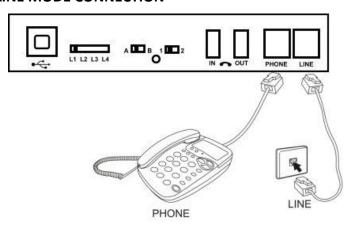
Disconnect the telephone line cord from the base of your telephone (the other end connects to wall socket) and plug this into the Universal Adapter 3.0 "Line" port. Connect the long cord supplied between the Universal Adapter 3.0 and the socket on your phone (where you removed the line cord). NOTE: The Universal Adapter 3.0 will record calls when connected to the phone line, it is not required that the telephone be connected to the device.
